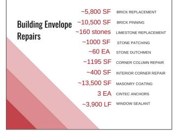
Figure 7: The repairs required to restore the building envelope
