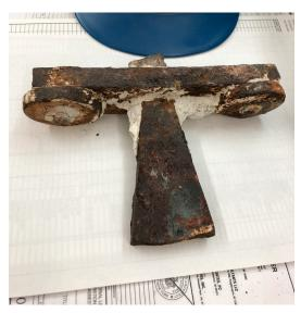
Figure 3: STN 500 stone lintel replacement in progress. Corrosion of the original dovetail anchor contributed to the formation of large cracks within the lintel.
